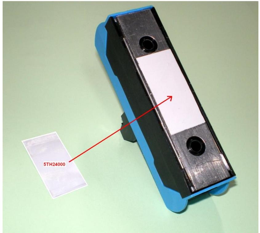
These thermal PAD with very good thermal conduction have also an electrical conduction. So all the mechanical parts stay connected to the earth. With some silicone thermal PAD the earth conduction is not achieved
