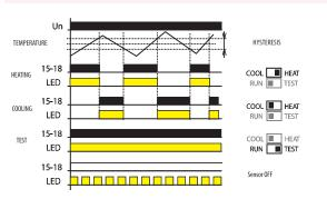
TER-3 It is a single but practical thermostat with a separated sensor for monitoring temperature. The device is placed in a switchboard and an external sensor senses temperature of required space, object or liquid. Supply is not galvanically separated from the sensor. The sensor is double insulated. Maximal length of a delivered sensor is 12m. device has in-built
